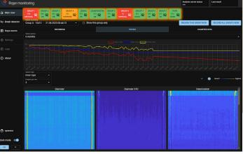
By leveraging trend analysis, the operators can visually track the rate at which ropes degrade over time in comparison to past occurrences.
