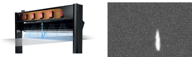
UV-Light Based Oil Inspection US Pat. 10,955,347
