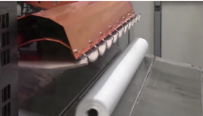
Tissue Log Roundness Analysis Log position, log diameter accuracy checking.
