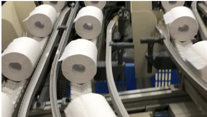
Tissue Roll Analysis The length of cut rolls, cut quality in the end of the roll, cleanliness of the cut, and ovality of the roll and the core checking.
